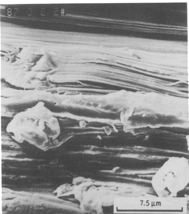
Figure 13 Lateral view of a bamboo-epoxy specimen showing slight buckling of bamboo fibres under compression.
